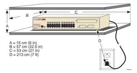
Figure 3-1 Tabletop or Shelf Installation
